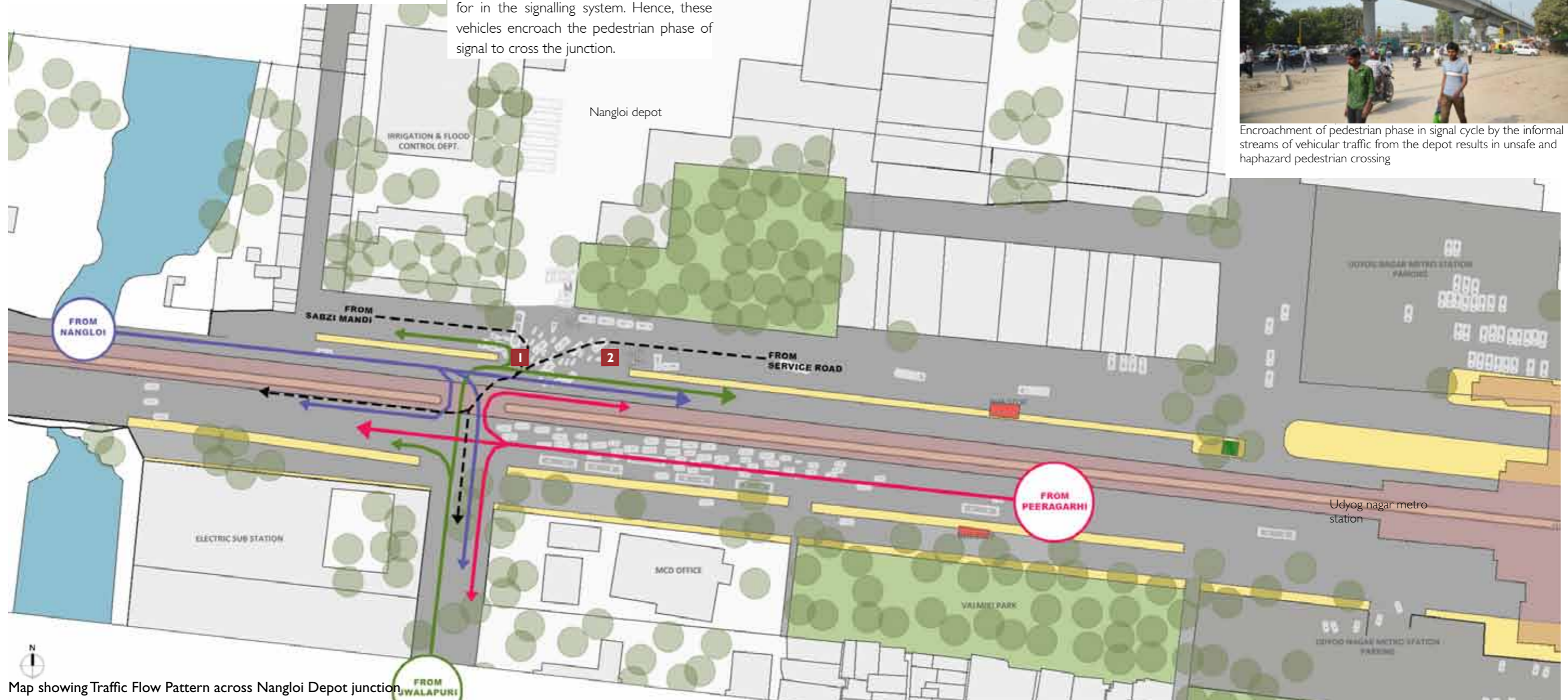
Flow diagram depicting different streams of traffic volume at Junction (in PCUs) from a sample survey carried out for 15 minutes
