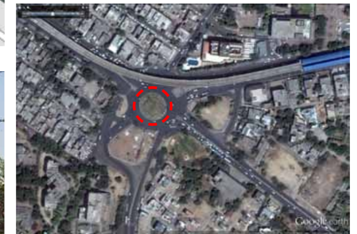
Time Line year: 2010 The roundabout was re-structured by adding another arm from Dr. K.S. Krishnan Marg. To manage the increased traffic and multiple traffic islands the roundabout was signalled.
