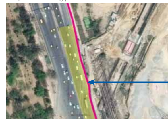
Inadequate merging length for traffic
