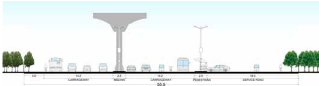
A - A' Cross section in front of Rail Neer Plant
