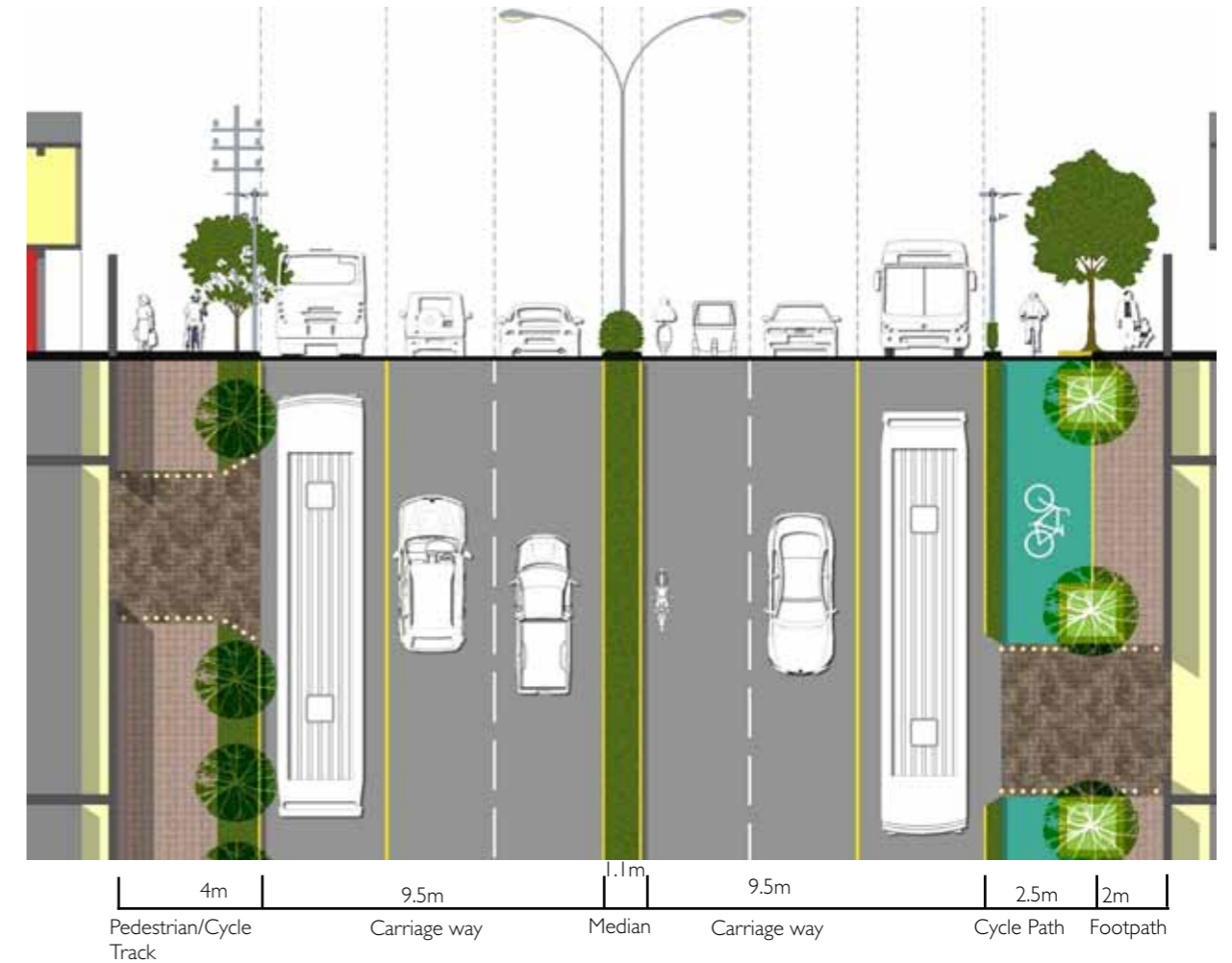
Section 02: Proposed section after Liberty Cinema
